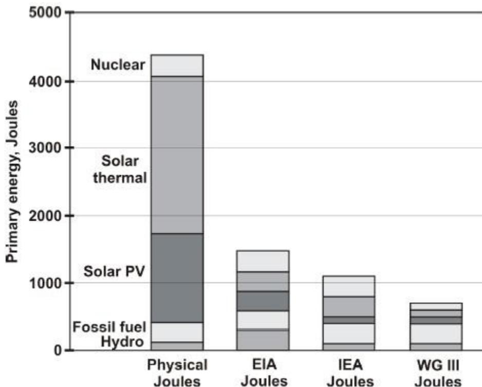
Figure 1. Graphical presentation of Table 2, primary energy to deliver 500 J of electricity.
